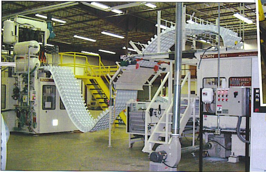
Above: The US method of forming and trimming separately — shown here on a Brown Machine system — is for larger production. Inset: Tool size is growing
